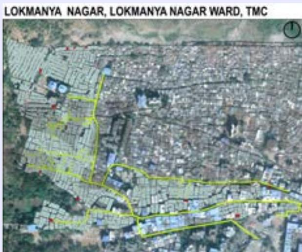
Fig 8. The map of the existing drainage line, Lokmanya Nagar.
