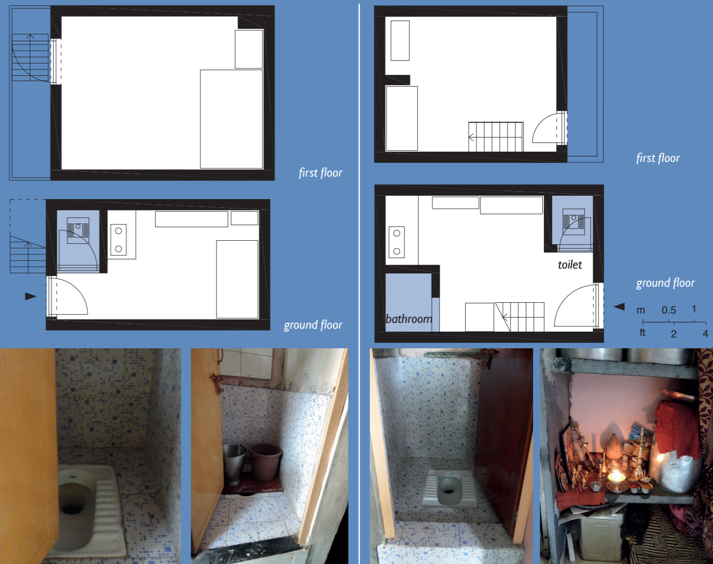
Illustration 1: In this house, 6 people live in 215 sq ft (20 m 2 ) on two floors. They needed to extend the existing bathroom structure of 1 ft (0.3 m) in order to build the toilet and bathroom. In order to use it as a bathroom, inhabitants put a board on the toilet pan, as illustrated in the pictures above.
